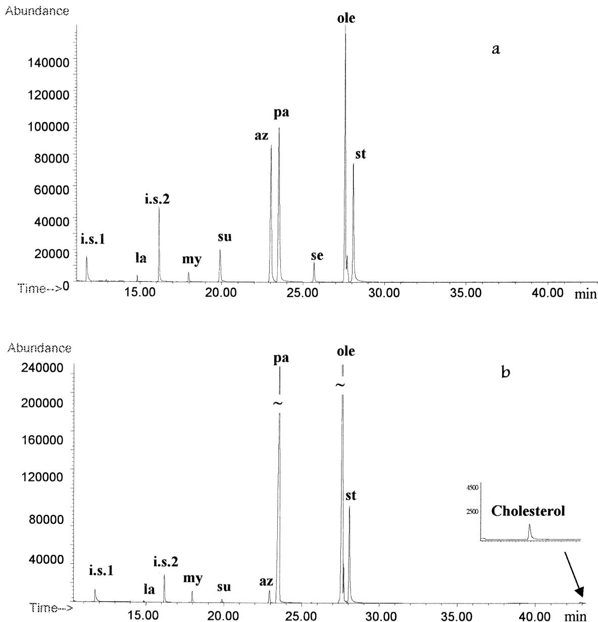
Fig. 2. Selected ion monitoring chromatogram of the derivatives of the fatty acid (a) from a sample containing linseed oil (1.0 mg), and (b) from a sample containing egg (1.4 mg).
