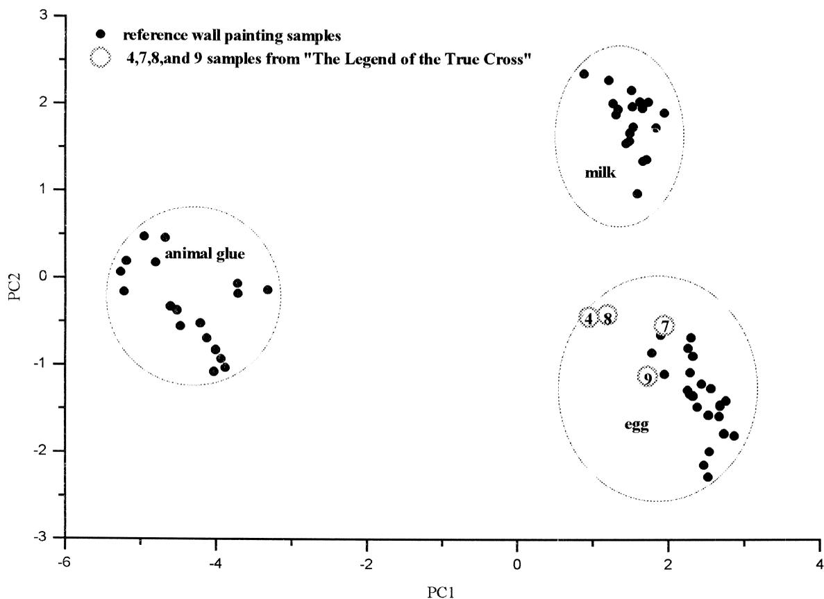
Fig. 5. PCA score plot of amino acid percentage data of reference samples containing egg, animal glue and milk binders (●) and of samples Nos. 4, 7, 8 and 9 from “*The Legend of the True Cross*”.
