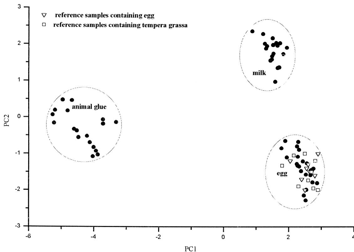
Fig. 3. PCA score plot of amino acid percentage data of reference samples containing egg, animal glue and milk binders (●) and of reference samples containing egg (▽) and “tempera grassa” (□) analysed according to the proposed procedure. Cumulative data variance on first two PCs 79%.
