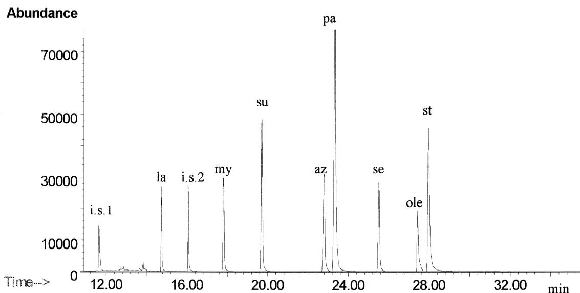
Fig. 1. Selected ion monitoring chromatogram of the derivatives of the fatty acid standard solution (injected amount: 1.5, 1.6, 4.5, 3.1, 9.7, 3.3, 2.5 and 5.7 ng. of la, my, su, az, pa, se, ole and st, respectively). Internal standards: i.s.1 hexadecane, i.s.2 derivative of tridecanoic acid.
